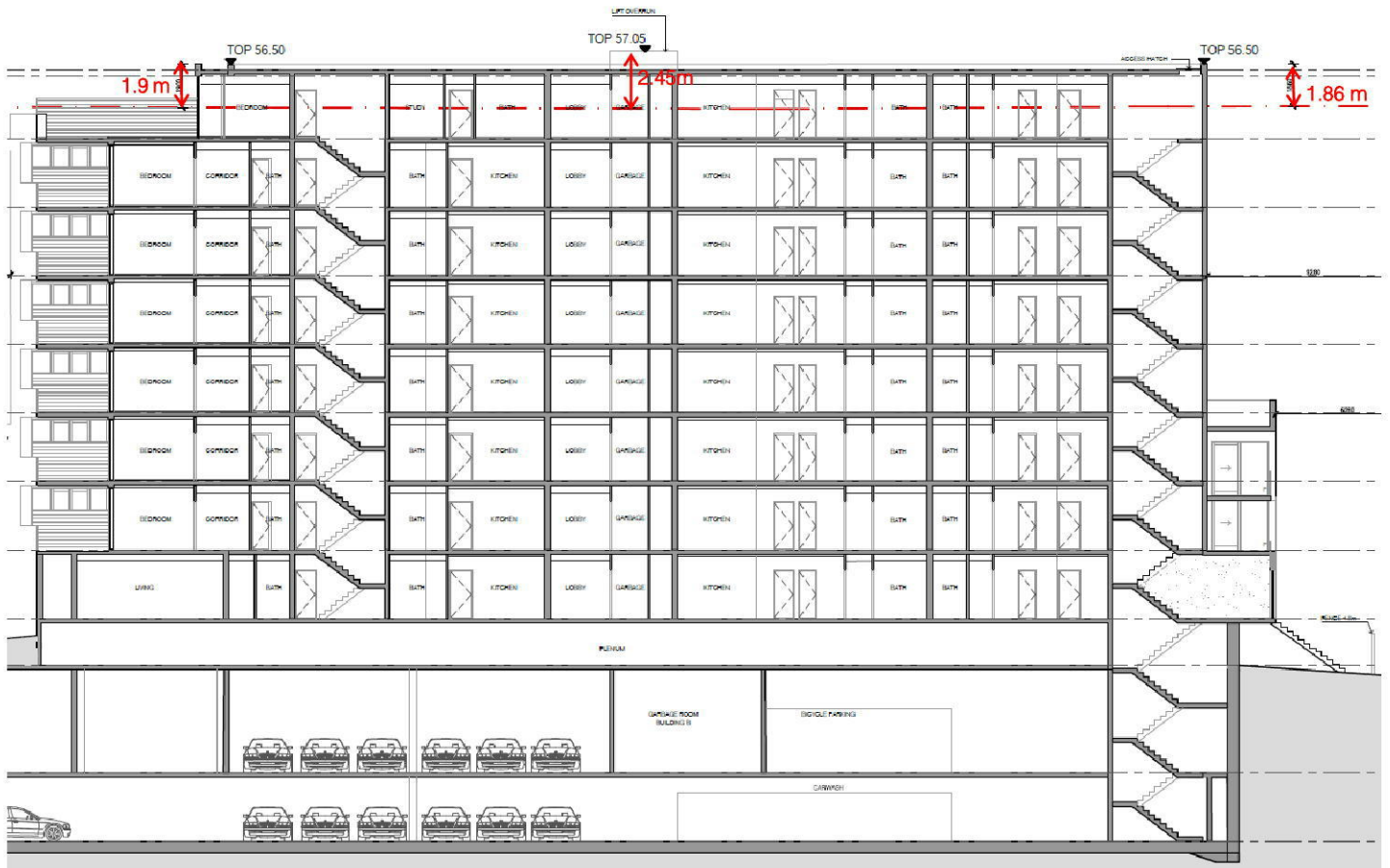
Figure 1: Example - Building B height non-compliance at section (Excerpt Section A-A)
